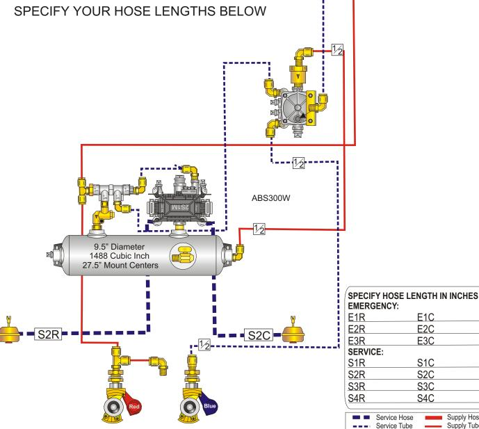
Hoses meet J1402 & JT106 specifications and are 3/8 ID unless otherwise noted. Reservoirs meet J10B specifications Pipe fittings are brass or plated SH80 steel. Push-in style 3/8 tube fittings standard. ABS Electronics pre-tested before shipment.
